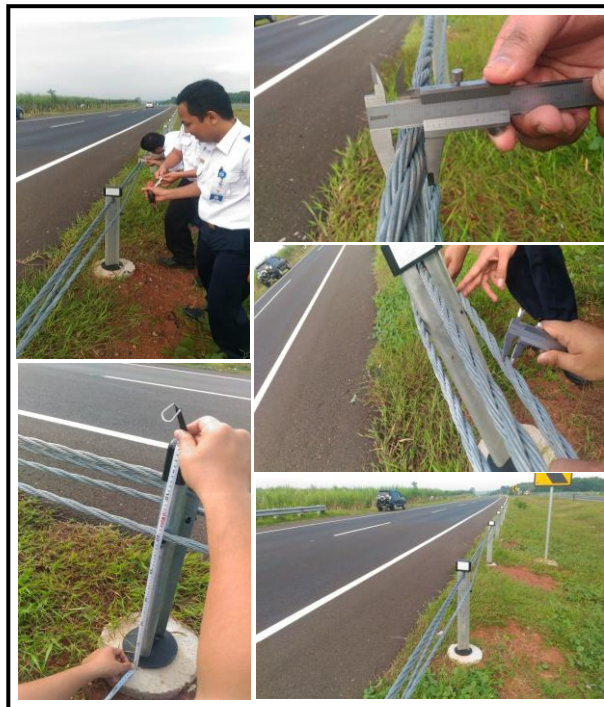
Gambar 7. Pengukuran Wire Rope di Ruas Tol Cipali.
