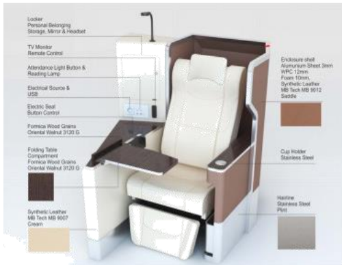
3D Rendering - Tampak depan final design enclosure sleeper seat
