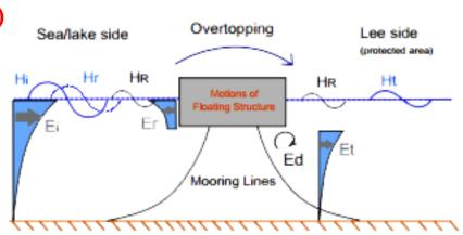
HR = radiated wave height Hi = incident wave height Hr = reflected wave height Ht = transmitted wave height Ei = incident wave energy Er = reflected wave energy Et = transmitted wave energy Ed = energy dissipation
