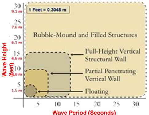
The general structure of the floating breakwater will function effectively in waters with a wave height below 5 ft or around 1.5 meter
