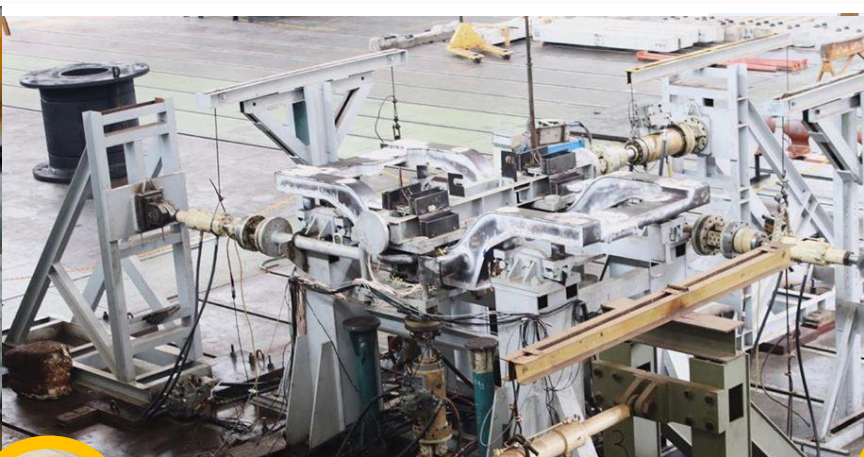
03 Structural Test of LRT-Jabodebek Bogie – B2TKS –
