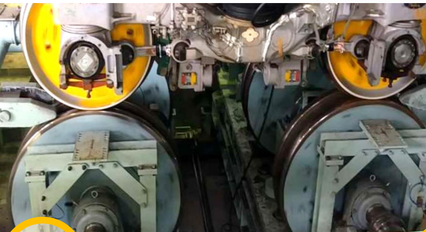
02 Bogie Full Scale Dynamic Test – Target 2022 –
